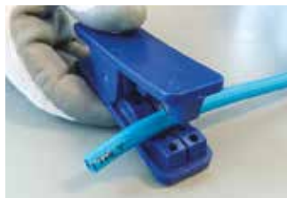
Tube cut at 90° with plastic tube cutter
