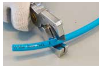
Correct tube cut with metal tube cutter
