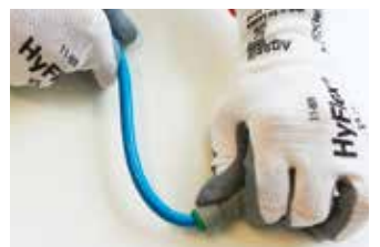
Fitting with tube inserted, having a tight bending radius
