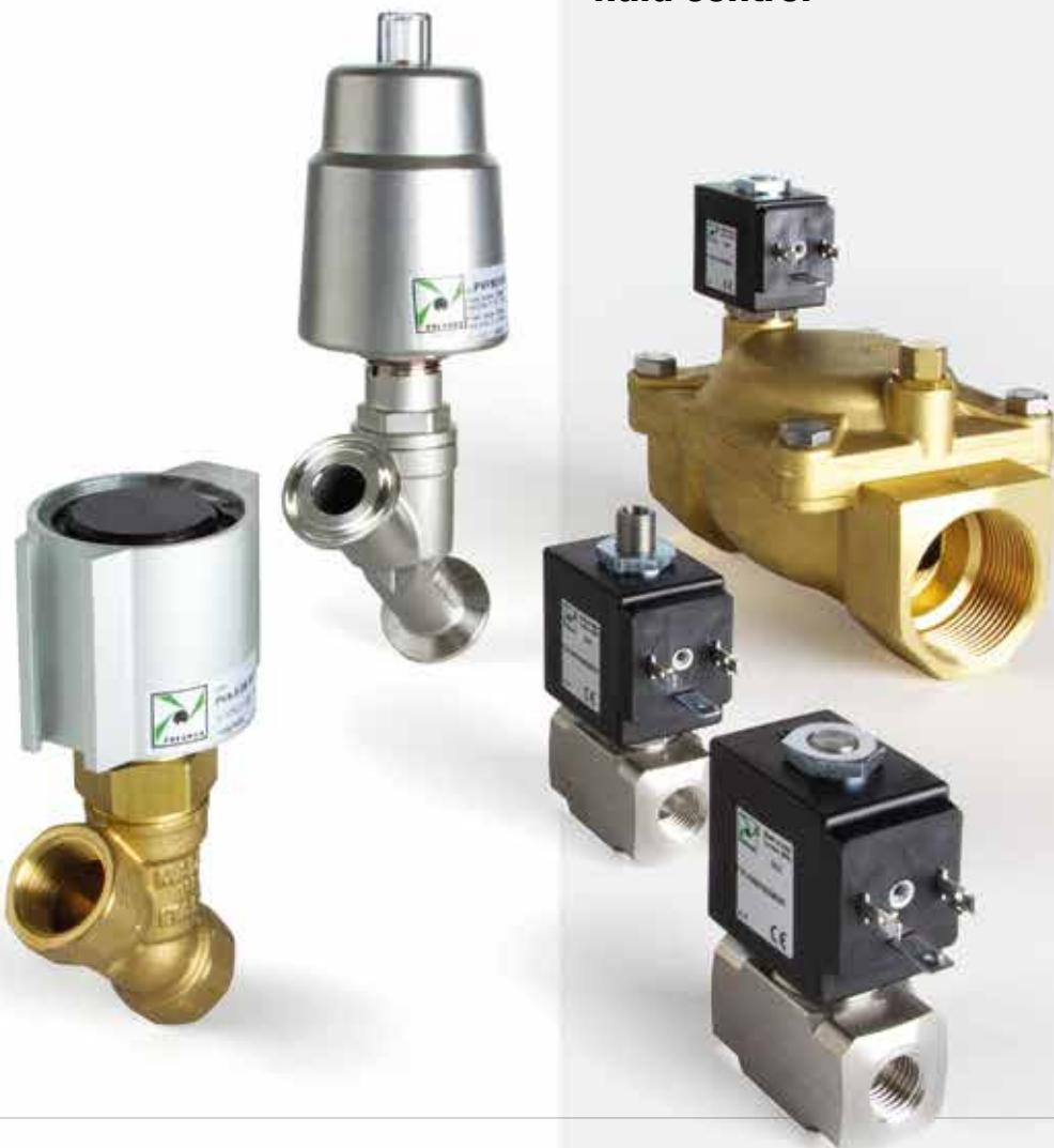
The Pneumax range of components designed for the control and management of liquid and gaseous fluids have been **manufactured considering suitable materials for the valve bodies (brass, stainless steel), internal components (stainless steel)** and seals (FPM, PTFE & EPDM) in order to guarantee maximum reliability even in harsh environments.
