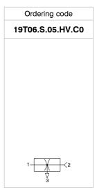
Single stage generators, with operation based on the Venturi principle; their main feature is the presence of feed pressure and connection for the vacuum on the same axis. This makes it possible to connect the suction cups directly to the generator or through the suction cup holder, so therefore still on the same axis with advantages in terms of system layout and simplicity.
