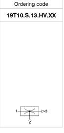
Single stage generators, robust and reliable, with compact dimensions and suitable for applications which need the required degree of vacuum to be reached quickly with limited air flows. Operating on the Venturi principle they have the vacuum connection orthogonal to the axis of supply and outlet. They can be connected directly to the suction cups and/or suction cup holder and applied in any position.
