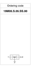
Single stage generators, robust and reliable, with compact dimensions and suitable for applications which need the required degree of vacuum to be reached quickly with limited air flows. Operating on the Venturi principle they have the vacuum connection orthogonal to the axis of supply and outlet. They can be connected directly to the suction cups and/or suction cup holder and applied in any position.
