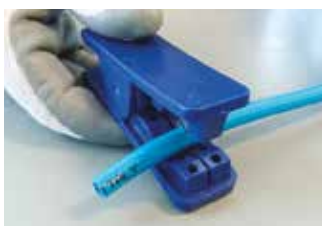
Tube cut at 90° with plastic tube cutter
