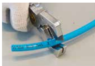
Correct tube cut with metal tube cutter
