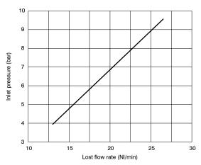
For higher drying efficiency, use the highest possible inlet pressure, even if this results in an increase in regeneration air.
