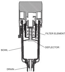
In the bottom of the bowl there is a device which is used to drain the particles which have been extracted from the air. This device can be automatic or manually operated, in case of the manual version it is important to ensure that the condensate level does not reach the deflector as it would be sucked back into the air line.
