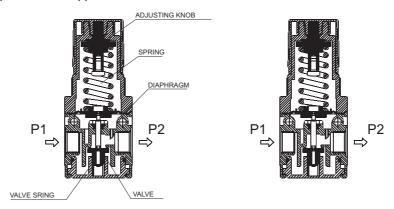
Compressed air pressure, both in reservoir and pipe lines, is continuously subjected to variation and fluctuation caused by inconsistencies in consumption and by irregular operation of compressors. Therefore, it is always necessary to regulate the air pressure in order to reduce it to the required values and to level it to a more constant supply.
