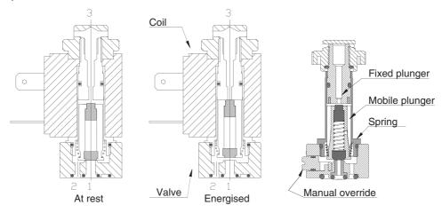
**Indirectly operated valves**: these valves are fitted with adirectly operated valve which upon receipt of an electric signal, actuates a pneumatic operator.
