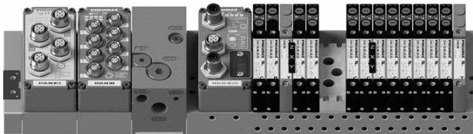
Example shown: 31-P-C4-D8-M12-E-C-B-T-XYZ-A-I-W-(2)C-XYZ-(6)C-T Manifold with external feeding, serial node, M8 input module, M12 output module; solenoid valves, multi-position diaphragm plugs, additional power supply module.
