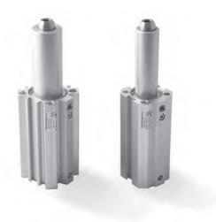
The swing clamp cylinder has been developed to meet the need to clamp a workpiece by means of a clamping arm which when released would unclamp rotate 90 degrees in order to allow unrestricted access to the workpiece; the stroke of the swing movement is 21mm.
