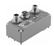
For each fieldbus node, maximum deliverable current by OUTPUTS  $+24\,\text{VDC}$  supply is  $4\,\text{A}$ , moreover the sum of the currents on OUTPUTS + 24 V DC and INPUTS + 24 V DC must not exceed 4 A.
