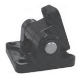
Mounting consists of clevis 09 and counter clevis. Used to mount cylinders at a right angle to the plane to which the counter clevis is attached. Allows selfalignment of the cylinder rod under load with an oscillation of  $\pm\,60$  degrees
