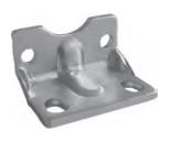
Elements used to anchor the cylinder parallel to the mounting plane. They are made of stamped and pierced sheet metal and painted in black. The mounting holes allow use with CNOMO, CETOP and ISO. Available up to 100 mm bore.
