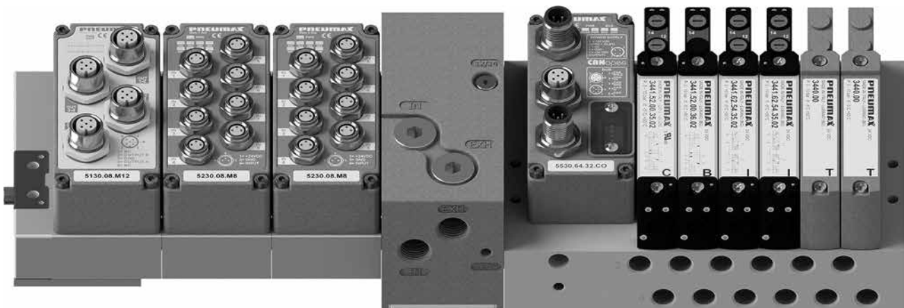
Example shown: 31-P-C4-(2)D8-M12-A-C-B-(2)I-(2)T Self feeding manifold with serial node, M8 input module, M12 output module, solenoid valves.
