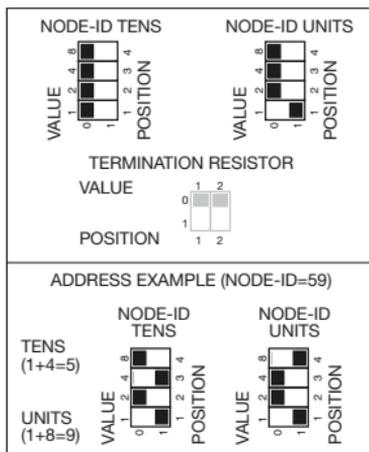
The device has a **built in termination resistor**. If the node occupies the last position in the network, the termination must be switched-on by moving the switch in position 1 (the switch is shown with light colour).
