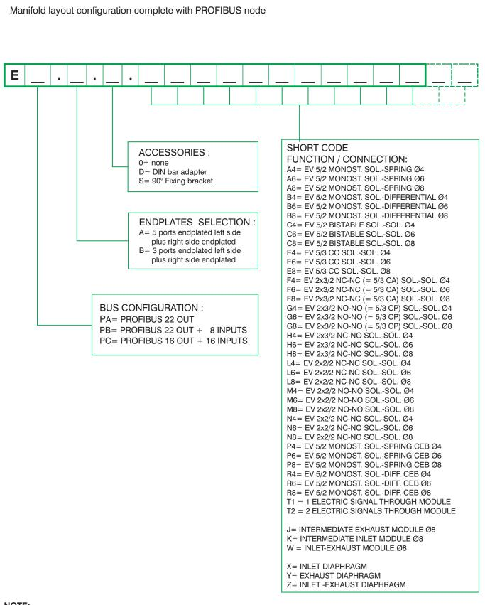
While configuring the manifold always bear in mind that the maximum number of electrical signals available is 22.
