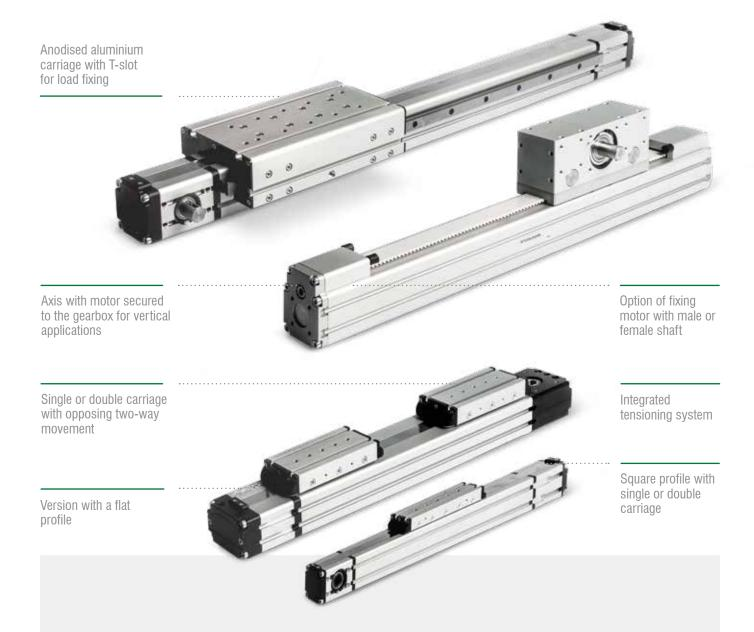
These linear actuators are equipped with a toothed belt made of reinforced polyurethane with steel strands and integrated tensioning system. They are available in the versions with one or two ball recirculating guide systems to support any type of load.
